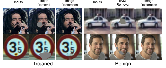
Figure 6: Image Restoration. Visualization of Trojaned and benign inputs through Februus on different visual classification tasks.
